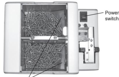
This inclined surface of each of the left and right inclined plates should be visible.
