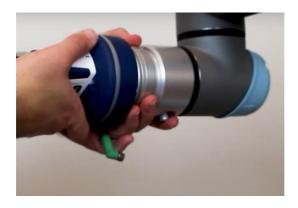
**Step 1:** Press the blue button on the male part all the way down.
