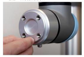
**Step 1:** Place the supplied Ø6 Dovel pin inside of the UR flange so that you can easily find the right position for the SpinMount.
