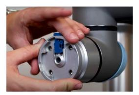
**Step 2:** Take the male part, align its holes with the holes on the robot and connect the part and the robot.
