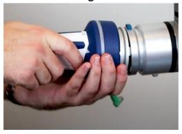
**Step 1:** Take the end-of-arm-tool with an attached female part and connect it to the male part in a way that the lines on the SpinMount and the male part connect.
