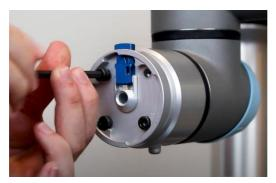
**Step 3:** Fasten the part with the 4 M6 screws that come in the package, using a hex key. The part should be well-adjusted, but pay attention to not fasten it too tight, as it can cause damage to the robot. Use 10 Nm tightening torque.
